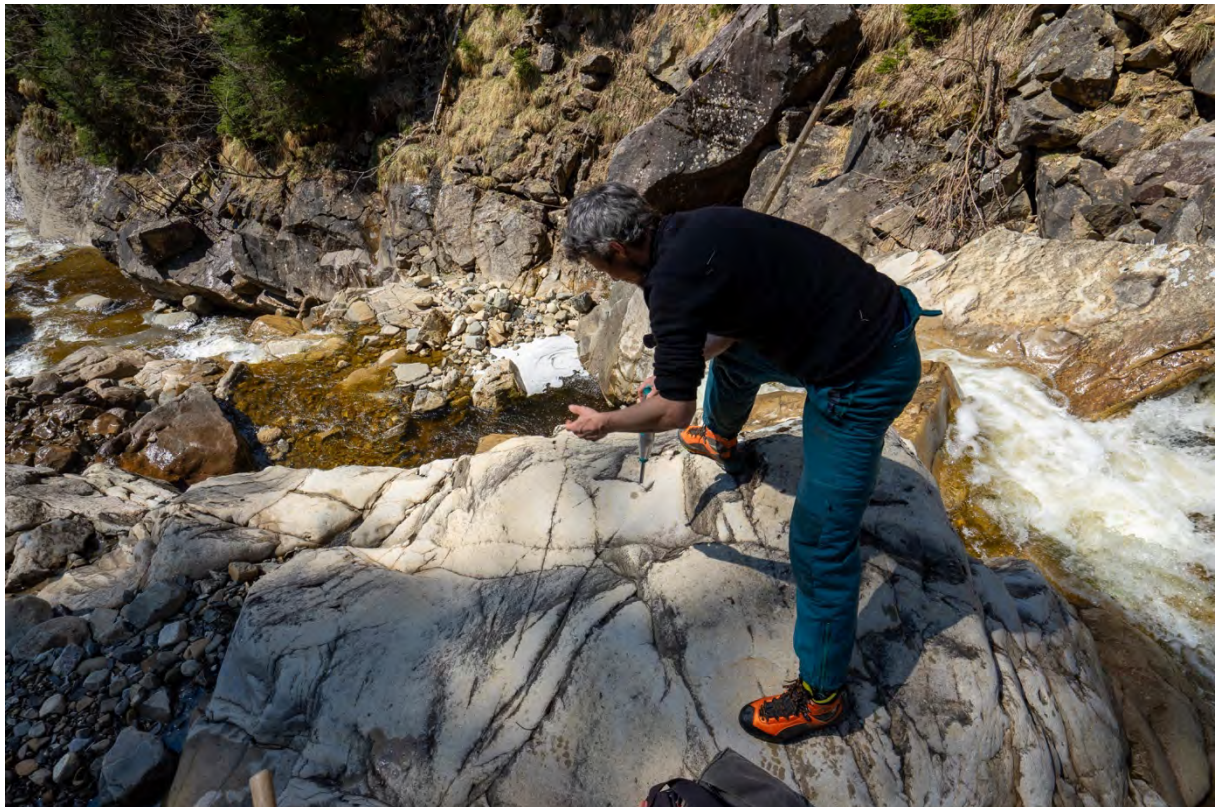
Fig. 5. Lukas Nibourel taking Schmidt Hammer measurements during field campaign as part of the hardrock aggregate units' project.
