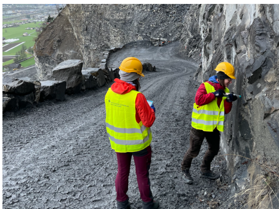
Fig. 2. Testing of the physical properties of the Altdorf Sandstone at the Attinghausen extraction site (1.4.2022).
