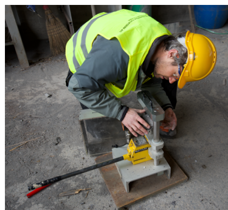
Fig. 2. Testing of the physical properties of the Altdorf Sandstone at the Attinghausen extraction site (1.4.2022).
